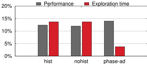
Figure 12. Performance and exploration time of the three different policies for an example mix of 3 applications ( bzip2 , libquantum and milc ). The time spent in exploration clearly has an impact on performance for some workload mixes.
