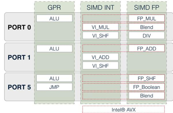
Figure 1. Execution cluster of Intel Sandy Bridge microarchitecture. Multiple operations are port-specific (e.g. FP\_MUL can only execute on port 0).
